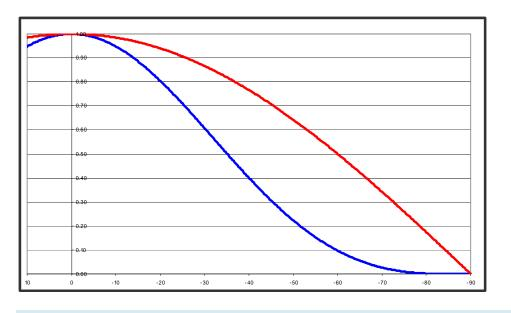
The red trace is the single LPFM antenna bay. The blue trace is the two bay half wave spaced antenna. At +/-70 degrees, the effective ERP of the station is 23 Watts using the single bay antenna.
